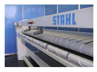
With the convenient clamp device it is possible to operate the SERVANT by just one person - even with large pieces of linen.
